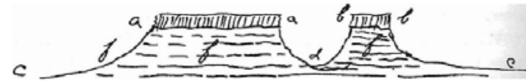
a-a and b-b, top of hill, level lava, very hard; c-c, plain; d, valley; f-f, soft strata of ashes lying under the lava.
