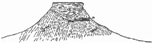
a, represents the lava top or "table"; b-b, the underlying gold-bearing slates, called the "bed rock," and also the "rim rock."
